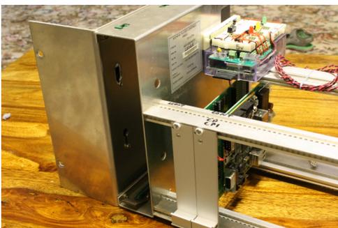
There are obviously a few other things that need to be done as well. A power supply and rack has been liberated from a redundant Tele 12 outstation, which helpfully provides both a 24v supply for the LIU and 5v for the RPI. Some breadboard, a few basic electronic components and a basic knowledge of electronics is all that is needed to wire the IO together. There is a weekend's work to learn everything you need, and pocket money to buy the parts, if you can't already find them.
